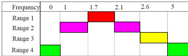
Frequency ranges (Hz) of the vertical and longitudinal vibration
