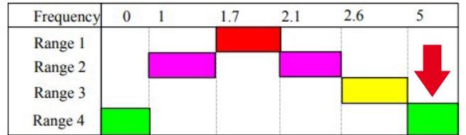
Frequency ranges (Hz) of the vertical and longitudinal vibrations
